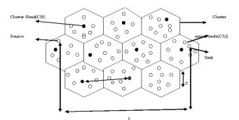
Fig.1. Cluster based End-End Multihop transmission
