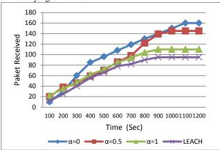
Fig.3. Comparison of data received by sink node
